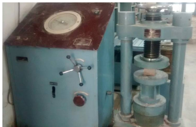
Figure 7: Compression Testing Machine
